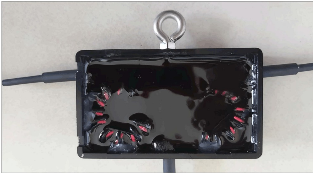
Fig. 7 - Inside the A-51 antenna matching unit
